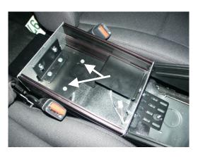
Attach rear floor filler panel (#6) to vehicle using OEM hardware
